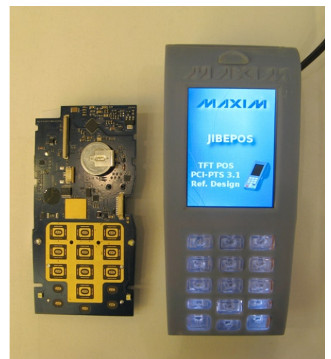
The NFC-enabled POS terminal reference design from Maxim, complete with its casing.
